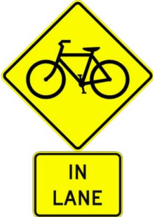
W11-1 with IN LANE plaque can inform users to narrow lane shared roadway conditions (TSMI 13-07).
