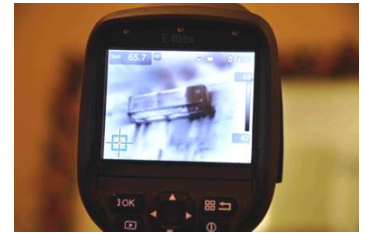
Thermographic cameras reveal air leaks that can be remedied with insulation.
